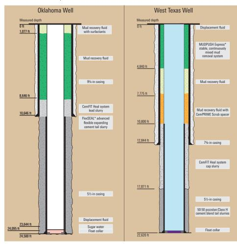
In Oklahoma, using a relatively small volume of CemFIT Heal system as a lead slurry cap maintained well economics while eliminating SCP.
