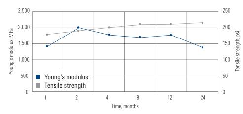
High-temperature aging data for FlexSTONE HT technology measured at elevated temperature for 2 years demonstrates stability with no degradation of mechanical properties such as Young's modulus (flexibility) and tensile strength.
