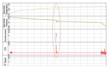
Real-time detonation indication (in oval) showing pressure, temperature, and CCL confirmations. The system also allows for postdetonation data download from downhole accelerometers showing shock.
