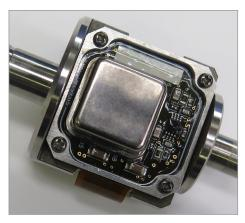
Solid-state MEMS technology means the GyroSphere service can withstand the rigors of drilling operations, including shock and vibration.
