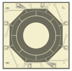
The GyroSphere service uses an internal vibrating structure to ascertain planetary rotation relative to the sensor.
