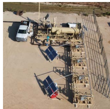
Four Vx Spectra flowmeters being tested head-to-head against a test separator.
