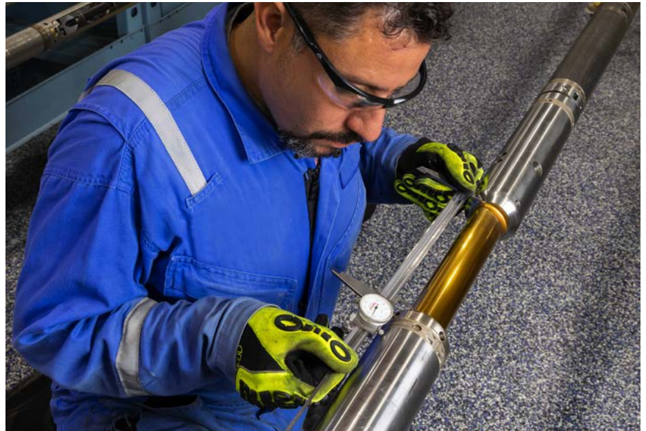
The ReSOLVE machining tool leverages the ReSOLVE anchor-linear actuator and ReSOLVE milling tool, delivering greater control and real-time measurements.
