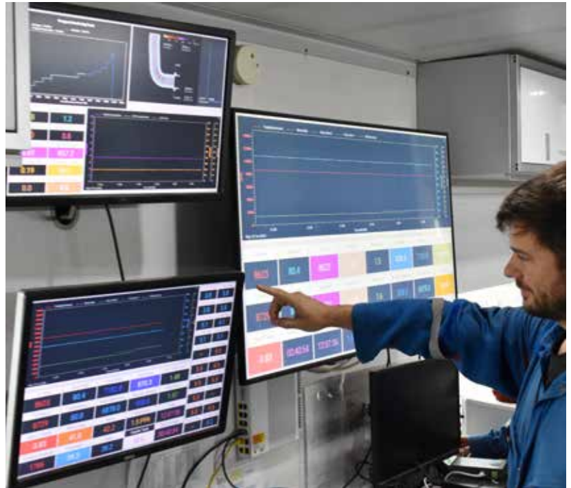
The FracCAT-X system's real-time displays, plots, and wellbore animations present a clear picture of the treatment as it occurs.
