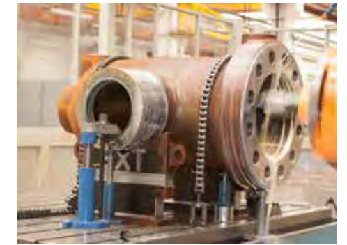
Gate valve forged body machining operations.
