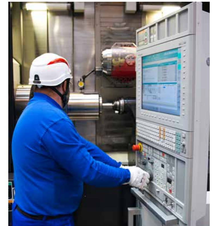
CNC operations on a chemical injection metering valve manifold.
