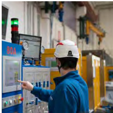
One of the seven automated small-bore valve test benches capable of 30,000-psi hydraulic testing and 20,000-psi gas testing.
