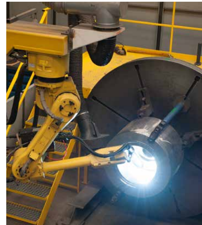
Robotic cladding process on a ball valve body.
