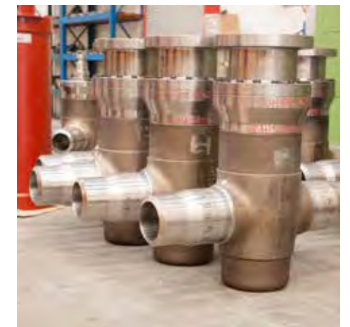
Final assembly prior to painting operations.
