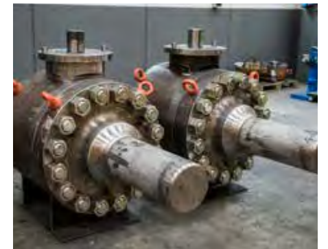
RING-O 10-in, 7,500-psi side entry ball valves.
