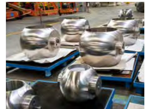
Valve components waiting for QC before installation.
